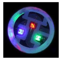
Tri-color LEDs contain three different LED emitters in one case. Each emitter is connected to a separate lead so they can be controlled independently. A four-lead arrangement is typical with one common lead (anode or cathode) and an additional lead for each color. Others, however, have only two leads (positive and negative) and have a built-in electronic controller.
