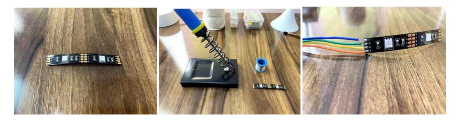
After fixing the two LEDs next to the dedicated holes for the light to come out of the inner C, I temporarily closed the entire rig with tape to test it out. But as it turns out the four wires needed to control the RGB LEDs hindered movement of the inner C within the outer C. Hence I had to switch to yellow LEDs because of their thinner wires.
