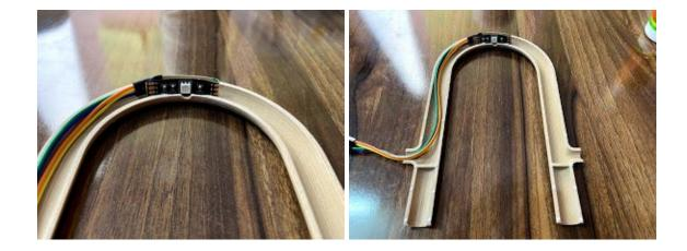
I took measurement of the insides of the inner C and temporarily fixed the light wire on the inside. I folded the wire in a neat fashion ensuring a good amount of LEDs near the two holes and then I blacked out the rest of the LEDs with electrical tape to ensure there is no excess light which might cause issues in the final long exposure photos.
