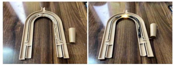
Then I temporarily closed the rig with tape while ensuring the wire attaching the LEDs with the battery enclosure going through the dedicated hole in the outer C. Then I fixed the battery enclosure with the outer C. After attaching the rod with the outer C, I tried out the mechanism and the inner C was moving freely within the outer C and everything was working as intended.
