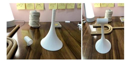
After putting the steel bearings in the housing inside the inner C as counterweight and covering with the caps I assembled the rest of the parts of the rig properly with feviquick.
